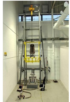
Fig 6: Photograph of a typical drop tower test fixture
